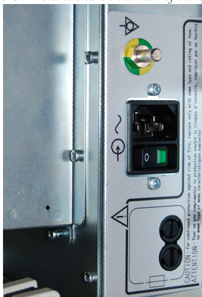
Fig. 3-3: Main switch on the rear of the system
